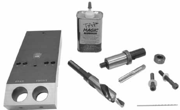
Jims Compression Release Valve Tool Use this tool for machining all TC 1999-on heads for preparing heads to install Jim's compression release valves. Install on the front or rear head, with or without the valves installed. Simply drill, spot face, tap and install compression release valves. 31586
