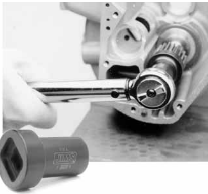
Jims Pinion Gear Nut Socket Use to remove or secure pinion gear nut to pinion gear shaft. 1/2" drive. Use with locker tool #31541. 31461 BT 1955-99
