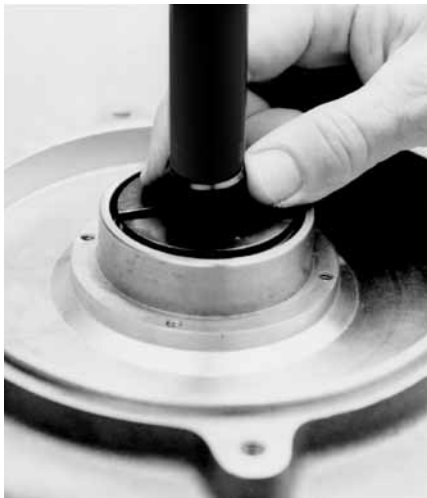
Jims Tool Driver Spacer Spacer applies outward force on the bearing race tool to grip the race better, allowing easier removal of race. Use with driver tools #31437, #31459, etc... 31557 Use on all bearing race tools
