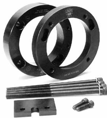
Jims Cylinder Torque Plates These plates simulate stress conditions when boring and honing. Correct torquing sequence is lasered on surface. Can be used on Screamin Eagle big bore cylinders. 31518 All Twin Cam to 4"
