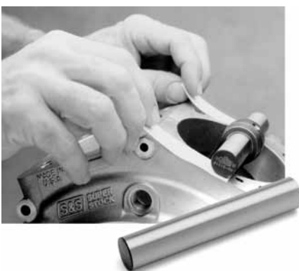
Jims Rod Alignment Tool Use to check rod straightness without removing rods from case. The alignment tool is 4-1/2" long. 31436 BT single cam only, including S&S and aftermarket motors
