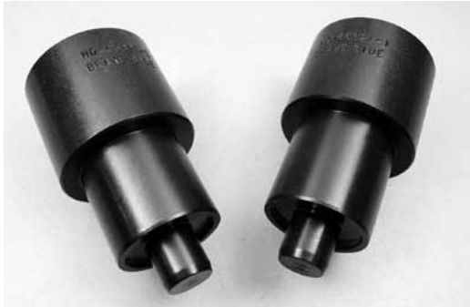
Swing Arm Bearing Installer Tool Use this tool to install both right and left swing arm bearings squarely on their bores to the installed depth on 2002-on FLT models. Replaces 45327. 26166
