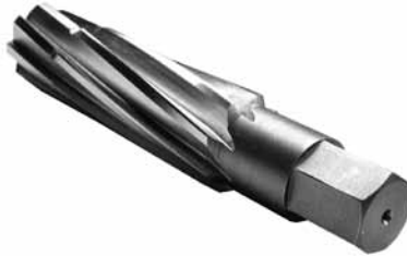
Jims Wrist Pin Bushing Reamer Use with rods in or out of motor. Use to ream wrist pins to HD specifications. Reamers are made to exact tolerances and piloted to locate from the I.D. of the newly replaced wrist pin bushing. 31548 Twin Cam
