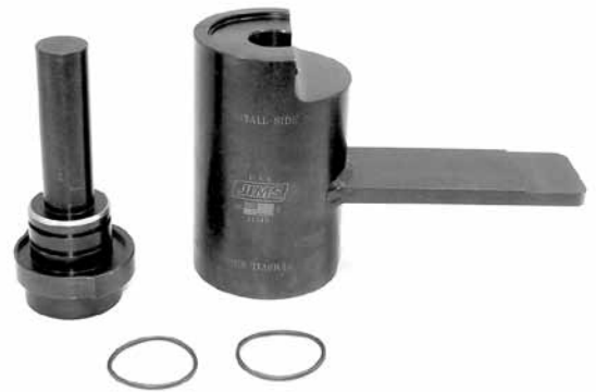
Jims TC Crankshaft Bearing Installer and Remover Designed to protect expensive engine cases by using a specially designed support block to remove or install cam side crankshaft bearing. Use press fit lube on case and bearings while installing. 31565
