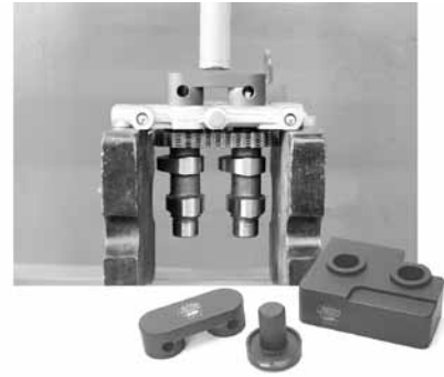
Jims Camshaft Remover and Installer Use to remove and replace front and rear camshafts and ball bearings in Twin Cams. It provides the precision alignment of the camshaft to ensure a smooth press in and out of the support plate. 31511 All Twin Cam
