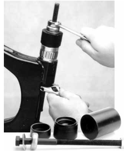
Jims Cleveblock Bushing Assembly Rear Swing Arm Tool Use to remove and replace swing arm cleveblocks. Cleveblocks are silicone filled bushings that will be damaged if not installed properly. Jims tool presses on the outer sleeve of the bushing, preventing damage to the cleveblock. Can be used with or without a press. 31564 Use on FLT 1980-on, FXR 1982-94 and all aftermarket FXR style frames
